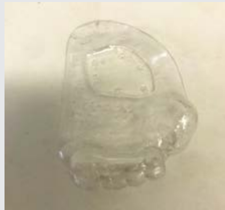
Figure 4 — The mouth guard manufactured by thermovacuum forming process
