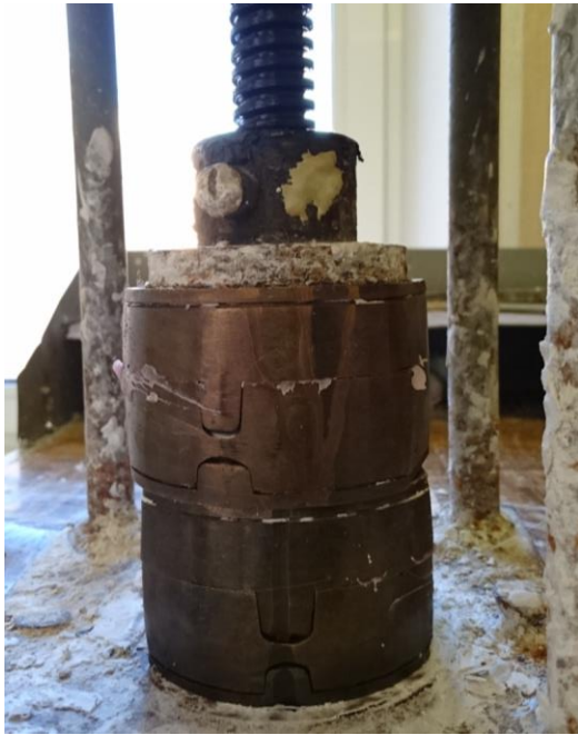
Fig. 63. Flask under the press for extruding plastic
