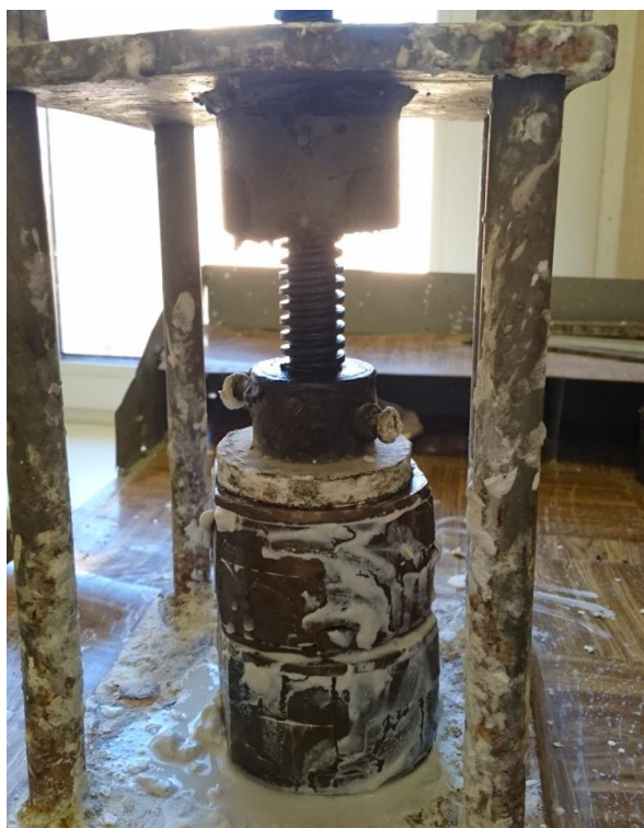
Fig. 54. Installation of the bottom of the flask and filling it with gypsum
