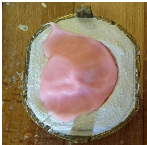
Fig. 62. Packing the plastic dough into the mold of the flask
