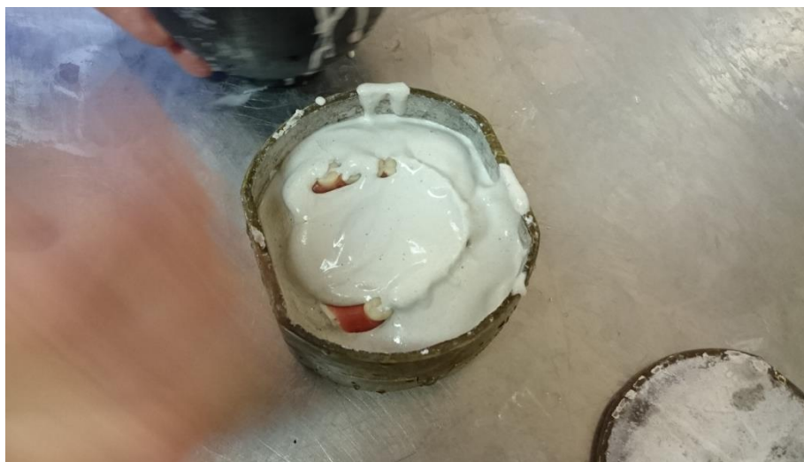
Fig. 54. Installation of the bottom of the flask and filling it with gypsum
